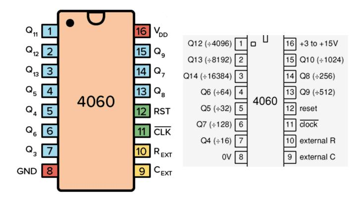
Similarly pin Q12, will undergo a change from low to high every 4096 (2<sup>12</sup>) cycles of the oscillator and is therefore diving the oscillator frequency by 4096.
