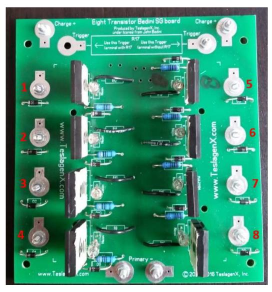
Radiant mode, 12mm gap, Battery LA1 (Flooded)@input, Battery A (AGM)@output, 7 power coils. Input +/-1.5amp Probe 1: x10, ground to negative of input battery, positive to collector transistor 1 Probe 2: x10, ground not connected, positive to collector transistors 2,3,4,5,6,7
