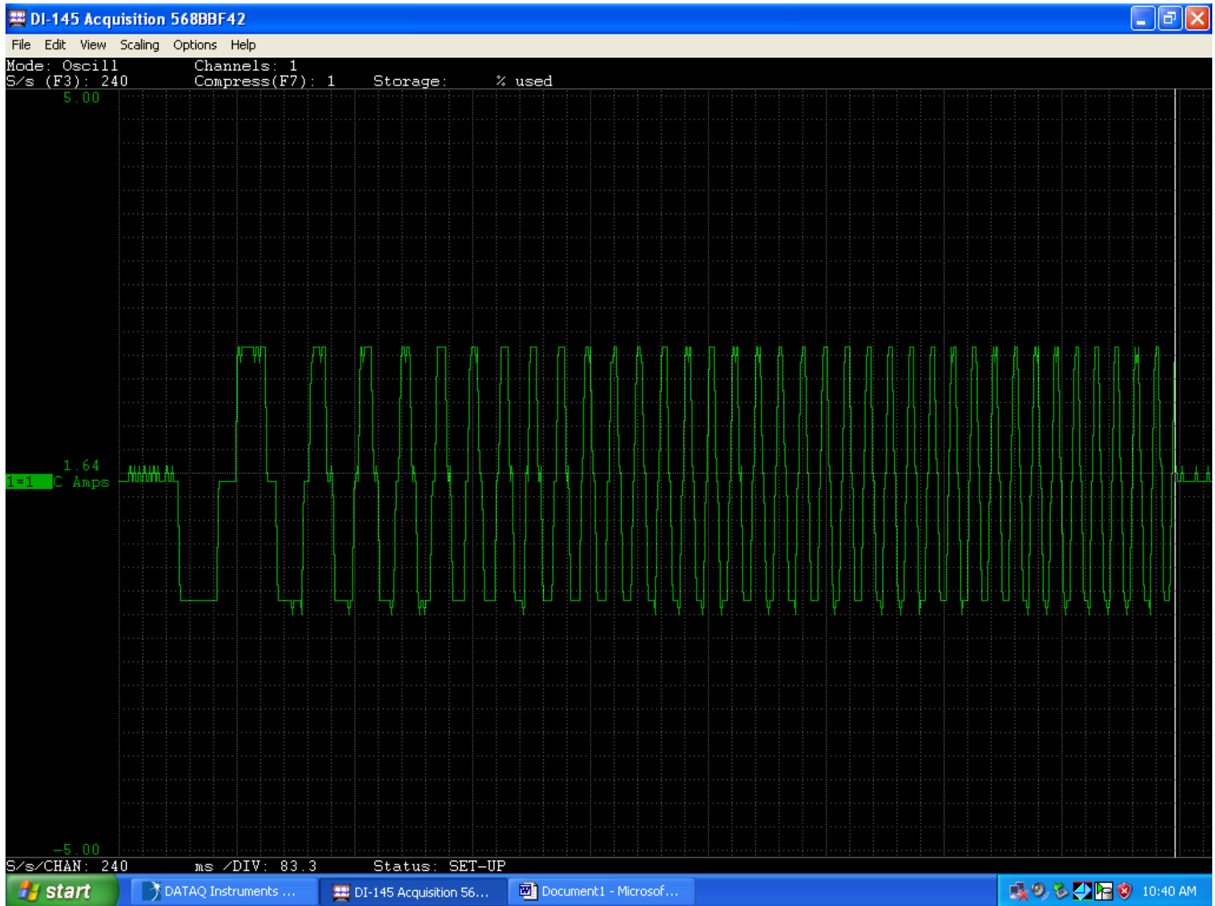
ZFM Proto Test Voltage vs RPM with reduced firing arc 55 degrees. 12 Volt test @ 500 rpm w/ 1.6 A 11/26/16 YIS Start-up Amps as motor accelerates
