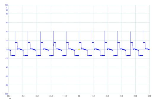
Scope measurement over 1 coil @ input (probe at 10x)
