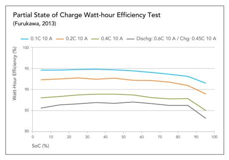
Figure 10: Results of efficiency testing undertaken at the Furukawa Battery Company (Furukawa, 2013)
