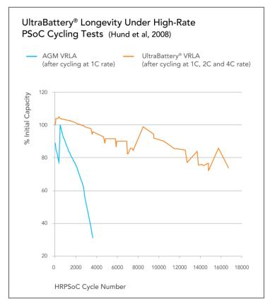
Figure 4: UltraBattery® longevity under earlier high-rate pSoC cycling tests (Hund et al., 2008)
