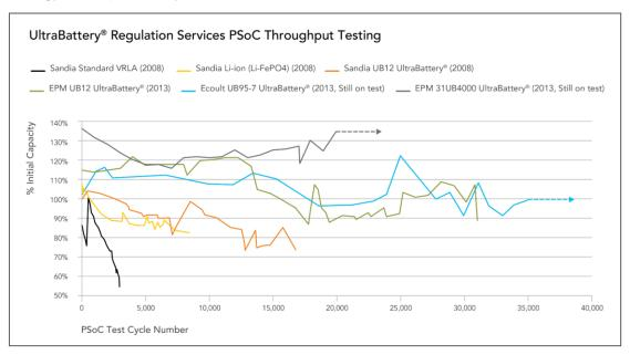
Figure 9: Energy throughput testing showing Sandia National Laboratories results from 2008 (lower three traces) for VRLA, UltraBattery® (UB12) and Li-Ion test results. The Sandia results are compared against internal testing carried out by Ecoult and East Penn Manufacturing (top three traces) performed in mid-2013. There is a clear trend toward increasing throughput as the UltraBattery<sup>®</sup> cells are improved over time.
