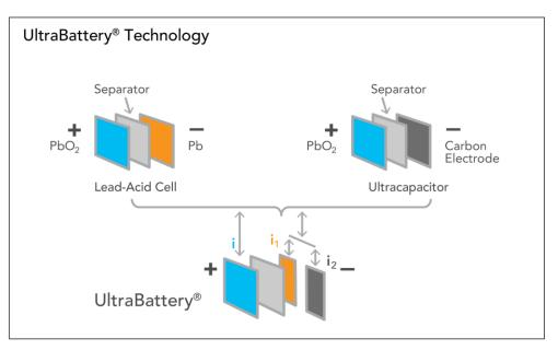
Figure 1: Schematics of standard lead-acid cell (top left), supercapacitor (top right) and their combination in the UltraBattery® cell (bottom)
