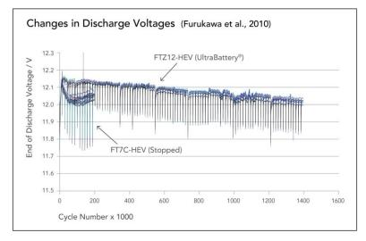
Figure 14: Changes in discharge voltages in individual batteries in 144 V strings of conventional VRLA and UltraBattery® cells under simulated medium-HEV cycling (Furukawa et al., 2010)
