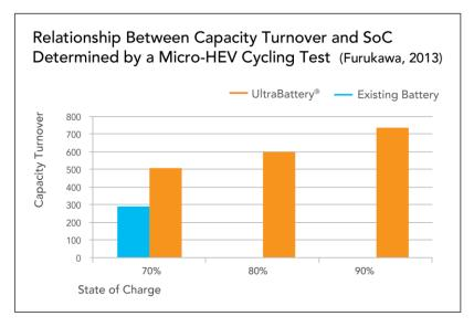
Figure 6: The relationship between capacity turnover and SoC determined by a micro-HEV cycling test (Furukawa, 2013)
