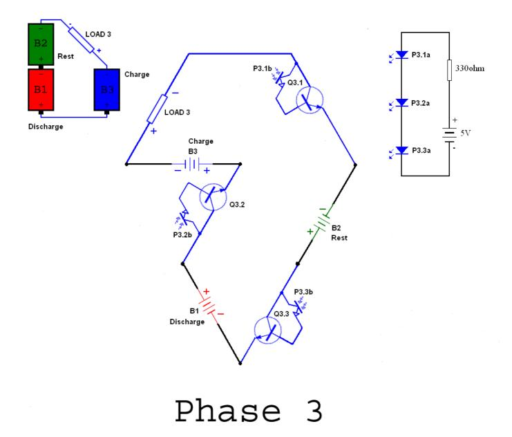
The switching cycles in the sequence of (Phase 1), (Phase 2) and (Phase 3)
